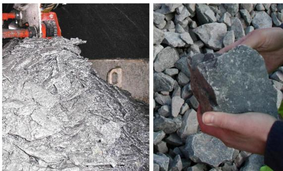
*Figure 14: The normal form of the excavation material in a regular way of the TBM operation (ships from tensile efforts) and the product places in the Hallandsås with numerous "cubic" pieces (from compressional efforts)*
